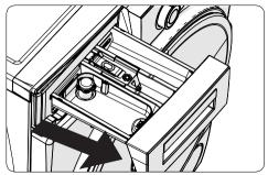
Press the region shown below inside the detergent drawer you have pulled all the way back, and continue pulling and remove the detergent drawer from its place
