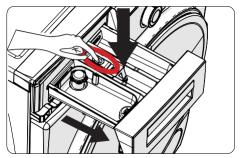
Remove the detergent drawer and disassemble the flush stopper. Clean thoroughly to completely remove any softener residue. Refit the flush stopper after cleaning and check that it is seated properly.
