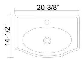
Dimensions of fixture are nominal and may vary within the range of tolerances established by ASME Standard A112.19.2.2013 Dimensions and specifications subject to change without notice.
