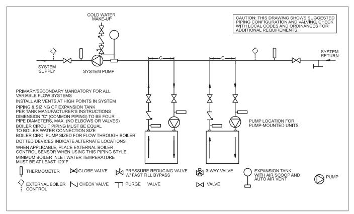
Figure 5. Hydronic Piping — Multiple Boilers, Primary Secondary System.
