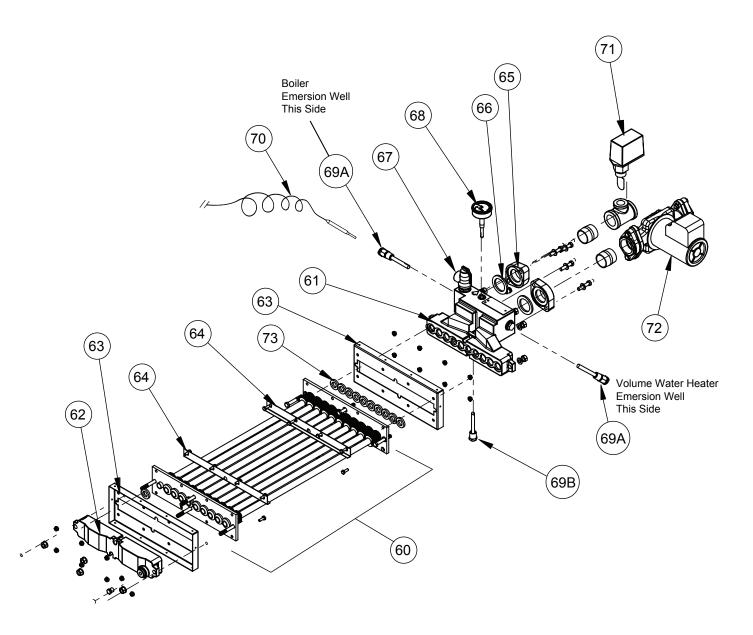
Figure 21. Heat Exchanger Components.
