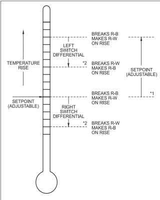
\*1 Difference between the temperatures at which the two switches make R-W. Adjustable from 3°F to 10°F (1.7°C to 5.6°C).
