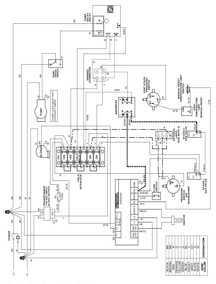
Figure 17. Wiring Diagram, Volume Water Heater.
