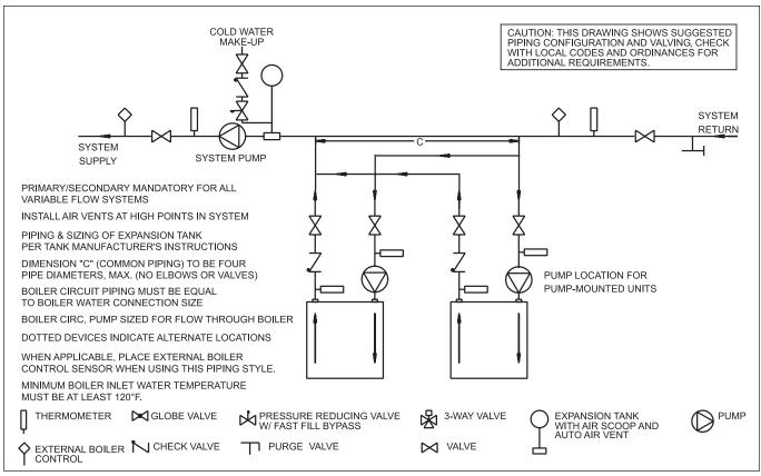
Figure 8. Hydronic Piping — Primary-Secondary, Reverse-Return.
