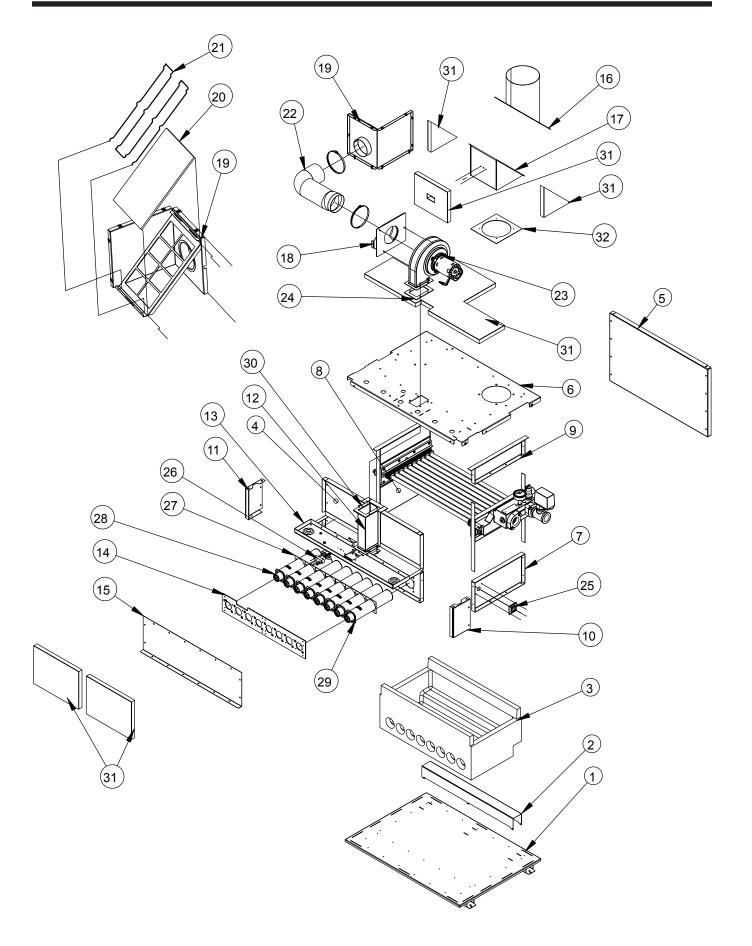
Figure 19. Combustion Chamber Components.
