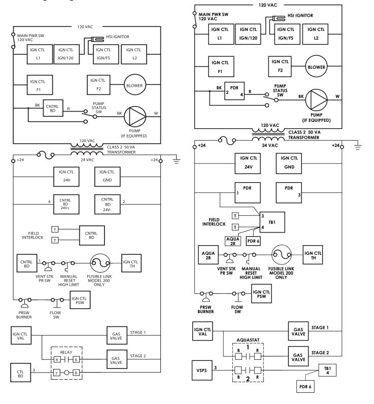
Figure 14. Logic Diagram, Hydronic Boiler
