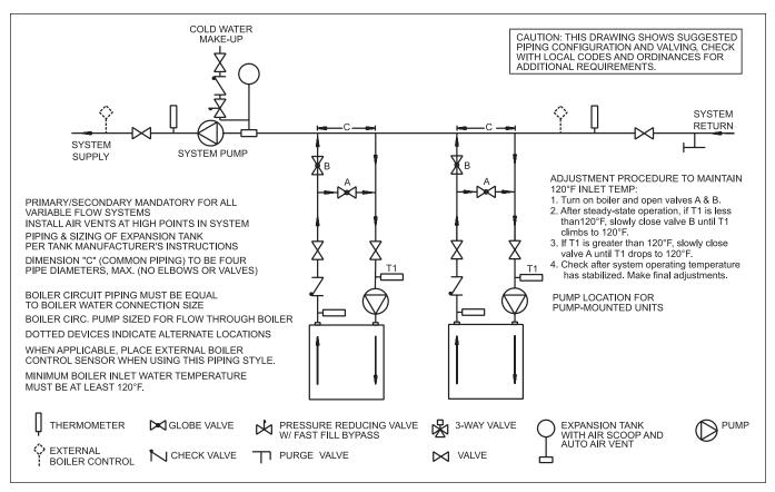
Figure 6. Hydronic Piping — Multiple Boilers, Low Temperature System.
