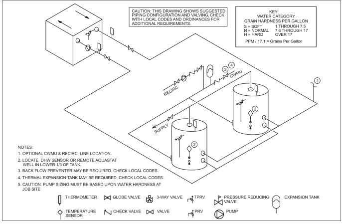
Figure 12. Water Heater Piping — One Heater, Multiple Tanks.
