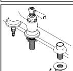
(3) For faucet with side spray, place side spray holder on mounting hole. Tighten locknut from underneath the sink to secure side spray holder.
