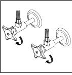
(1) Shut off the water supply. Remove old faucet. Clean mounting surface in preparation for new faucet.
