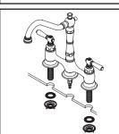
(2) Apply adequate plumbers putty along the boundary of base gasket. Align faucet with mounting holes and place faucet on the sink. Slide washers on shanks and secure the locknuts to the shanks from underneath the sink.
