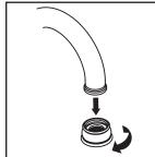
(5) When using stainless steel braided faucet supply hose; this faucet requires one end of the supply hose to have a 1/2" female IPS connection. The other end of this supply hose must match the thread on the water supply valve under your sink. Once you've identified the required size, carefully follow the manufacturer's installation instructions for each hose.
