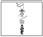
(4) Thread escutcheon with gasket from top of the side valve, attach handle to the side valve with help of 3/32" Allen wrench put hole cover on the handle. Place cold and hot side valves in position on the sink, ensure handles operate in correct direction. From underneath the sink, hand-tighten locknut to the side valve. Position side valve to desired location from top. Tighten screws on locknut with the help of Phillips head screwdriver to secure side valve.
