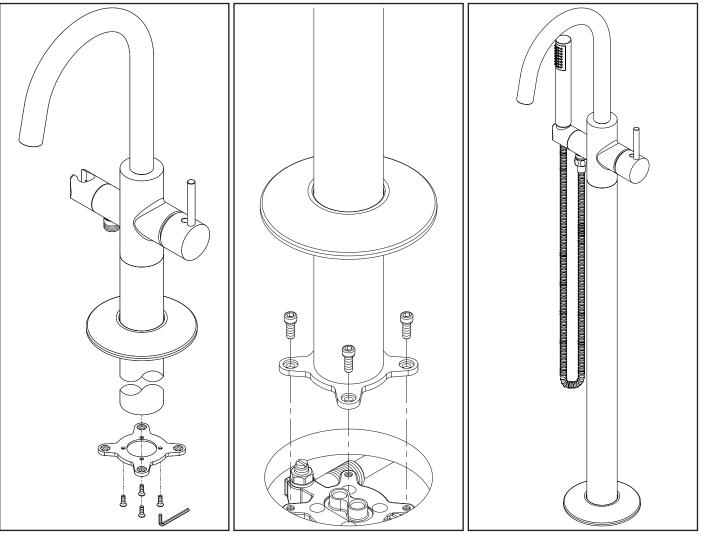
(1) Slide flange through the faucet body from the (2) Carefully align the two inlet copper tubes bottom of the faucet. Tighten the four screws to secure mounting bracket to the bottom of the faucet body by using a 3/32" Allen wrench.
