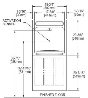
Note: New Installations Must Use Ground Fault Circuit Interrupter (GFCI). It is highly recommended that the circuit be dedicated and the load protection be sized for 20 amps.
