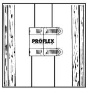
Slide Proflex coupling over the pain spigot ends of the two pipe.
