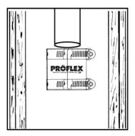
Loosen the stainless steel clamps. Clamps are riveted to the shield and will not remove.
