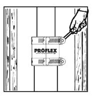
Tighten clamps to 60 inch-lbs. or torque.
