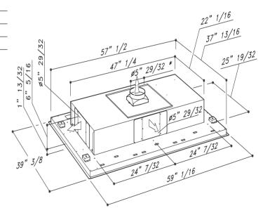
\* accessory outlet Ø8" For the installation, create a false ceiling with a niche of 57" 11/16 for 37" whose minimum height to be reached is 10" 5/8
