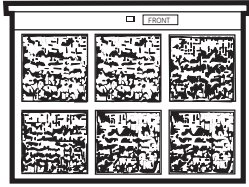
Dirty filter— Needs cleaning
