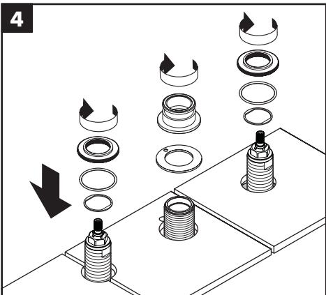
Install the stop rings and mounting rings on the valves.
