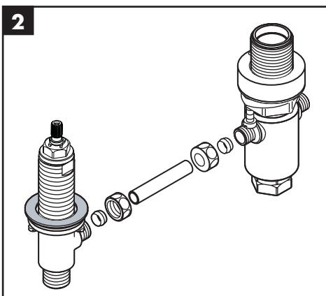
Connect the valves and diverter housing using the copper tubes and  $\frac{3}{8}$ " compression fittings.
