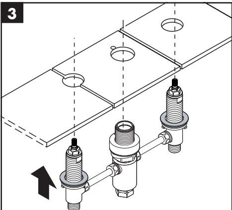
Place the valves and spout tee on the mounting surface.
