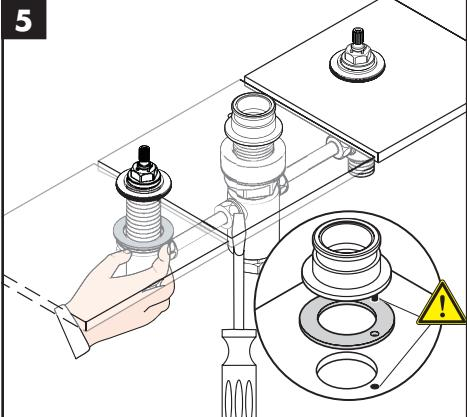
Rest the assembly on the mounting surface, with the spout adapter pin inserted in its hole.
