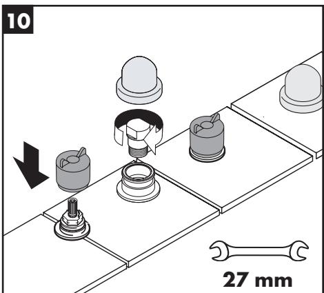
If the trim is not to be installed immediately, install the spout tee plug and the plaster shields.
