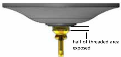
Drawing 2 Canopy Adjustment
