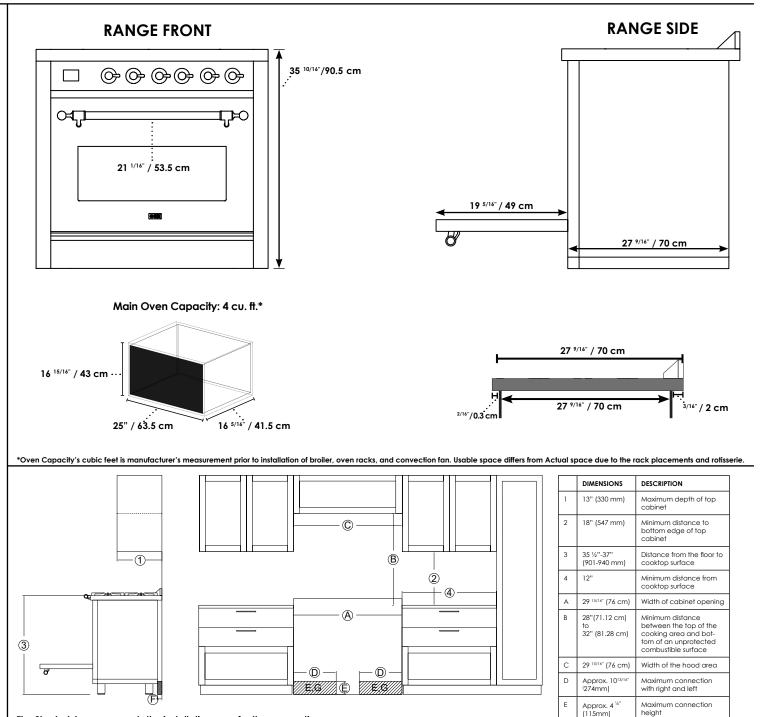
The Shaded Area represents the installation area for the connections; E; Electric Connection
