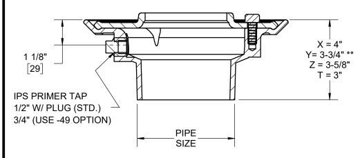
\*\* GASKET ON -Y CONNECTION CONFORMS WITH ASTM-C564
