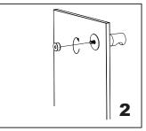
Screw in the fixing bracket into the knob bolt.
