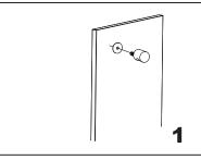
Install the knob (bolt) through the glass hole, make sure the rubber gaskets are between knob&glass.
