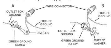
Make wire connections. Reference chart for correct connections and wire accordingly.
