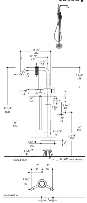
In-floor plumbing connections 2 x 1/2" copper pipe
