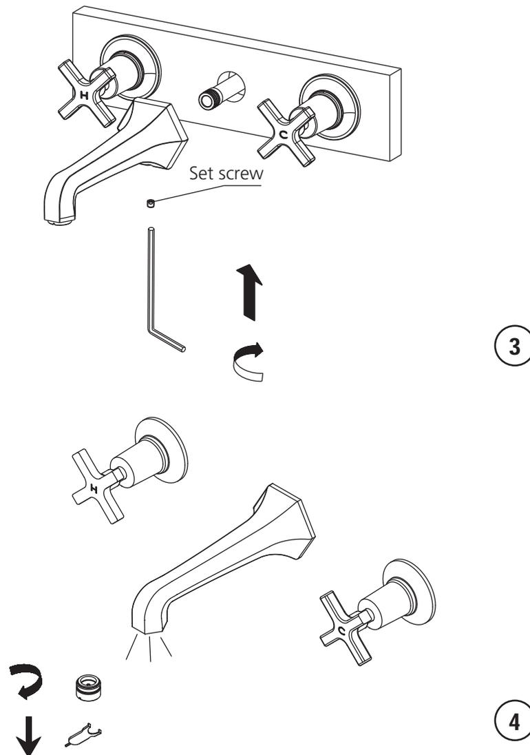
**3** Install the spout and fix it tightly with set screw.
