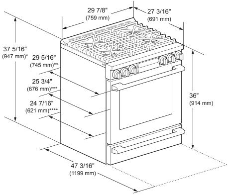
\*Including Grates (Unit can be raised an additional 1" (25 mm))
