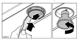
Insert the lever supplied into the gap between the bulb and the bulb holder.
