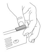
• Remove top plug/bushing from the door using a flat head screwdriver. Discard the bushing.
