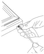
• Insert the new bottom plug/bushing in the new bottom of the door. Secure with the screw removed from the old plug/bushin.
