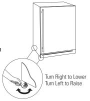
adjust the rear leveling legs approximately 1/8" less than the opening height. Screw front legs all the way in to shorten the height at the front. This will allow you to slightly tip the unit into the opening. Once in the correct position, the front legs can be adjusted to level the product.
