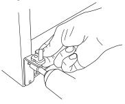
Remove the plastic cap from the top left corner of the toe kick and discard.
