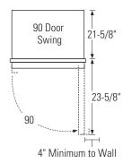
**NOTE:** Clearances are based on the recommended 2-1/4" handle standoff depth.
