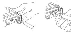
Install the bottom trim onto the new bottom side of the door.
