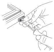
• To install the door, set the door onto the left bottom hinge pin. Holding the door in place, insert the new top left hinge pin into the door and secure the hinge to the case with screws.
