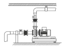
Fig. 21. Installing the pump
