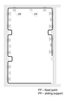
Fig. 18. Locations of fixing supports on horizontal distribution lines
