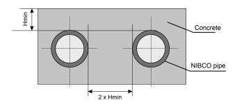
Place pipework to be covered with concrete in a location that will not be subject to damage during settlement of the building (e.g. due to cracking of concrete screed).
