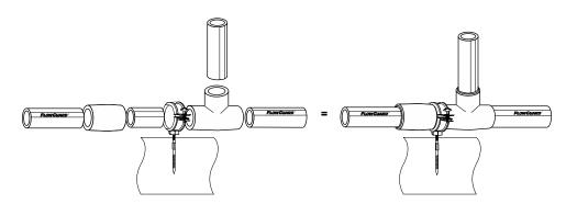
Fig. 16. Fixed support on pipe (using fittings)
