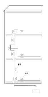
Fig. 17. Locations of fixing supports in service drop
