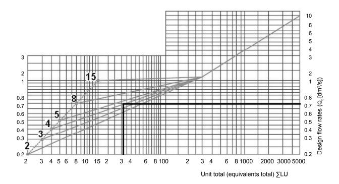
Fig. 1. Nomograph for determining design water flow rates in water distribution systems (Qo [dm3/s]), depending on the total of equivalent load units ( $\Sigma$ LU)
