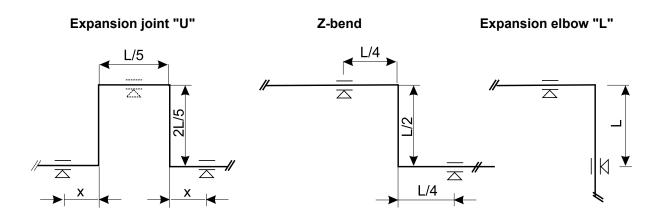
Fig. 6. Expansion joint types
