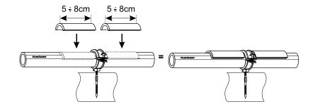
Fig. 15. Fixed support on pipe (using cement)
