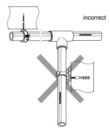
Fig. 14. Correct and incorrect inclusion of an expansion elbow
