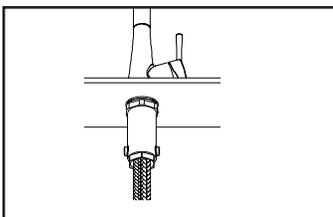
(4) From under the sink thread locknut to the faucet. Tighten the locknut with the help of supplied mounting tool.
