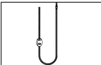
(5) Install the weight on the pull-down spray hose. Adjust the weight so that the pull-down spray head is retractable. Connect pull-down spray head hose to the outlet hose.
