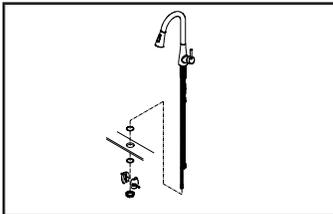
(2) **For 1-Hole Installation :** Install 1-Hole mounting assembly on the faucet. Ensure there is a washer under the faucet. Place the faucet in position on the sink.
