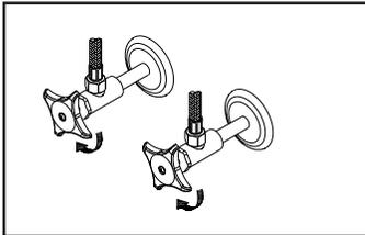
(1) Shut off water supply. Remove old faucet. Clean mounting surface in preparation for new faucet.
