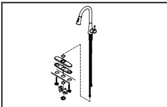
(3) **For 3-Hole Installation :** Install supplied deck plate underneath of the faucet. Apply plumbers putty under the base gasket. Place the faucet in position on the sink.
