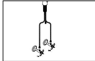
(6) Connect hot and cold inlet supply hoses to supply stops. For 1/2" connection use 3/8" male to 1/2" female adapter for installation. Adapters are optional and not provided with the faucet.
