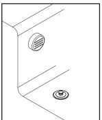
(5) Test to see if overflow cap is staying firmly on the adapter. Pull and push the strainer group for functionality.
