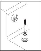
(3) Use a flat head screw driver and turn clockwise to attach the stopper onto the strainer at the bottom of the tub until tightened. Do not over tighten.
