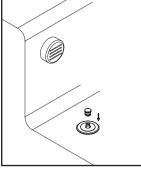
(4) Hold push & pull knob (d) to turn clockwise to attach onto stopper (c) until tightened. Do not over tighten.
