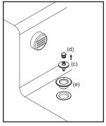
(2) For item OP-440065, Hold the push & pull knob (d) and turn counter-clockwise to detach from stopper (c). Plug (e), for -BN, -MB, & -ORB finishes only, onto the chrome strainer at the bottom of the tub.
