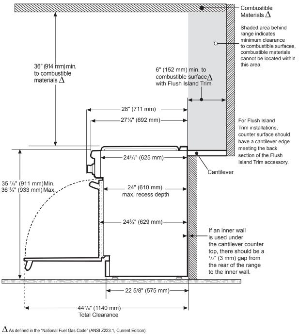
Clearances from non-combustible materials are not part of the ANSI Z21.1 scope and are not certified by CSA. Clearances of less than 6" (152 mm) must be approved by the local codes and/or by the local authority having jurisdiction.
