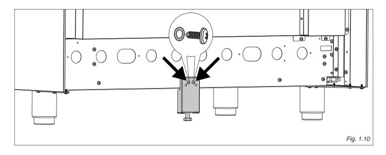
2. Fix the adjustable bracket to the back of the range (centered on the lower edge) using the two supplied screws and washers.
