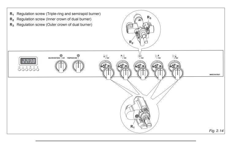
After regulation repeat the operations indicated in paragraph "2. PRESSURE REGULATOR" at page 13 and 17. If the range has been disconnected and then connected again to the gas supply line repeat the operations indicated in paragraph "5. LEAK TESTING" at page 17.
