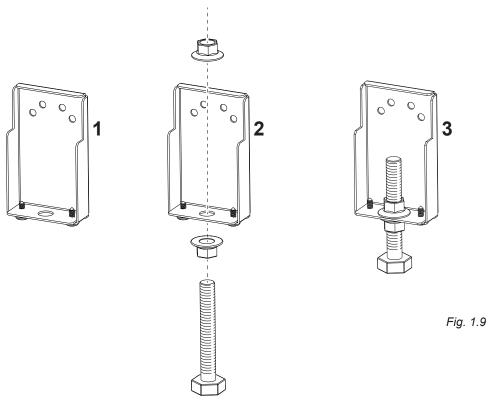
1. Thread the bolt through the adjustable bracket and fix in place using the two supplied nuts. Exnsure the nuts are well tightened.
