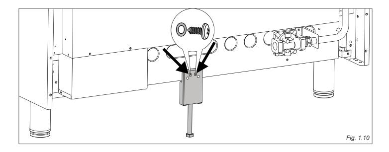
2. Fix the adjustable bracket to the back of the range (centered on the lower edge) using the two supplied screws and washers.
