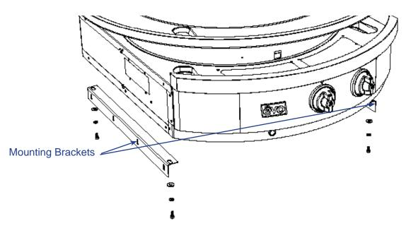
**STEP 6:** Remove two (2) mounting brackets with 7/16" Open End Box Wrench installed on Evo Affinity 25E Cooktop.
