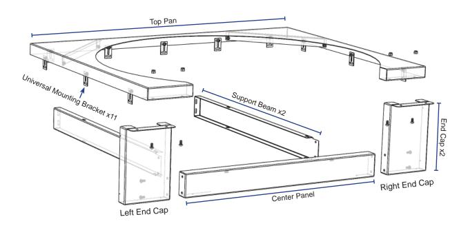
The Trim Kit for the Evo Affinity 25E is shipped partially assembled and requires installation and final assembly. Included in the kit are six (6) separate stainless steel metal components and one (1) package of hardware as listed below:
