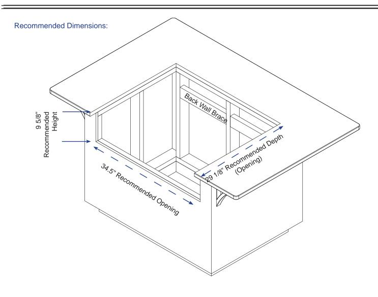
**STEP 1:** Prepare cabinet construction using either wood or steel framing. It is recommended to have a cutout measuring 29 1/8" depth by 34 1/5" width by 9 5/8" height.
