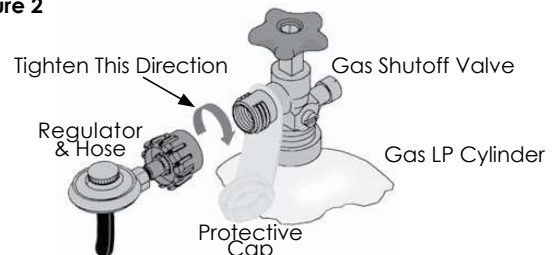
Quick Disconnect Hand-Wheel Regulator Install Figure 2
