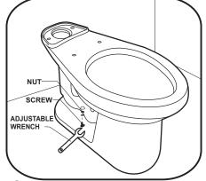
REMOVE TOILET SEAT FROM ITS BOX AND PLACE IT IN NORMAL POSITION ON THE TOILET FLANGE, WITH THE SCREWS INSIDE ITS BASE; BE SURE IT STANDS STRAIGHT. NEXT, PLACE THE NUTS AND SECURE THEM WELL WITH AN ADJUSTABLE WRENCH.
