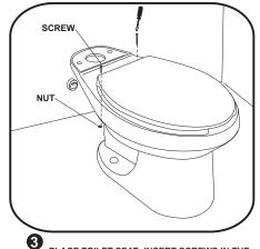
PLACE TOILET SEAT; INSERT SCREWS IN THE HOLES ON SEAT'S RIM; TIGHTEN SCREWS UNTIL IT IS WELL SECURED.
