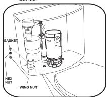
ONCE THE TANK IS PLACED ON THE BOWL, INSERT GASKET AND WASHER ON THE SCREW; ONCE INSERTED, TIGHTEN HEX NUT UNTIL TANK IS WELL SECURED; BE SURE NOT TO OVERTIGHTEN FOR IT COULD BREAK THE TANK.
