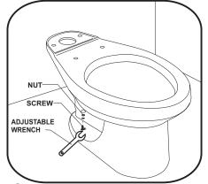
REMOVE TOILET SEAT FROM ITS BOX AND PLACE IT IN NORMAL POSITION ON THE CLOSET FLANGE, WITH THE SCREWS INSIDE ITS BASE; BE SURE IT STANDS STRAIGHT. NEXT, PLACE THE NUTS AND SECURE THEM WELL WITH AN ADJUSTABLE WRENCH.
