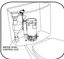
TO CONTROL WATER LEVEL IN TANK, TAKE BOLT AND TURN IT COUNTERCLOCKWISE TO DECREASE WATER LEVEL AND CLOCKWISE TO INCREASE IT.
