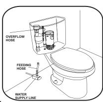
TO SUPPLY WATER TO THE TOILET USE A FEEDING HOSE, WHICH HAS TO BE CONNECTED TO THE WATER SUPPLY LINE IN THE FLOOR.
