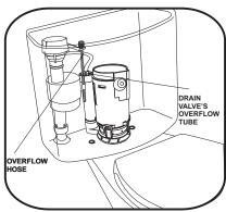
TAKE OVERFLOW TUBE AND THE BASE TO FIX
