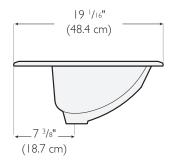
A.D.A. Lavatory Installation Requirements: Lavatories shall be mounted with rim/ counter surface no higher than 34 inches (86.4 cm) above finished floor. Provide a clearance range of 27-29 inches (68.6 - 73.7 cm) from the floor to the lavatory bottom or lavatory apron depending upon de type installed. For complete details on installation requirements, see A.D.A. Installation Handbook.
