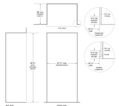
NOTE: 3<sup>1</sup>/2" (89) finished returns will be visible and should be finished to match cabinetry Shaded line represents profile of unit.
