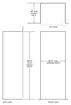
NOTE: 31/2" (89) finished returns will be visible and should be finished to match cabinetry Shaded line represents profile of unit.
